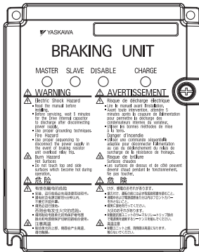
Figure 2 Warning Information Position
