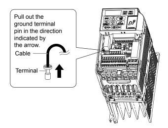
Figure 7.7 Pull Out the Ground Terminal
