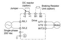
Figure 3.3 Connecting Single-Phase Main Circuit Terminals
