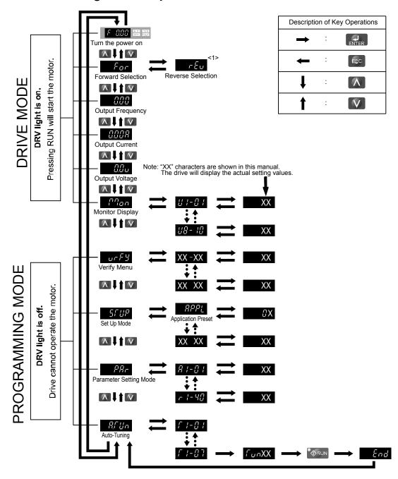
Figure 4.3 Digital LED Operator Screen Structure
