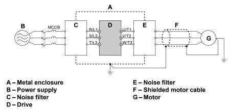
Figure 8.9 Reducing Radio Frequency Noise
