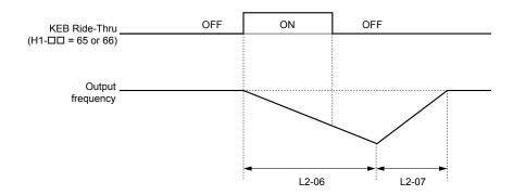
Figure 5.80 KEB Ride-Thru Timing Diagram for Multiple Drives
