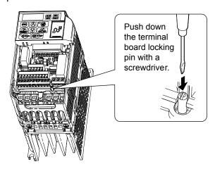
Figure 7.8 Depress the Plastic Tab
