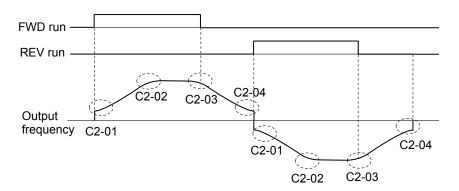
Figure 5.28 S-Curve Timing Diagram - FWD/REV Operation
