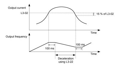
Figure 5.83 Stall Prevention During Acceleration for Permanent Magnet Motors
