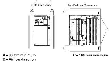
Figure 2.2 Correct Installation Spacing
