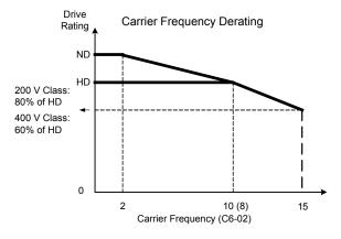
Figure A.1 Carrier Frequency Derating
