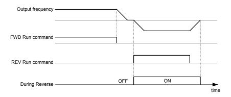
Figure 5.66 Reverse Direction Output Example Time Chart
