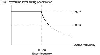
Figure 5.84 Stall Prevention Level and Limit During Acceleration
