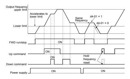
Figure 5.49 Up/Down Command Operation
