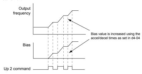
Figure 5.40 Up/Down 2 Bias when d4-03 = 0.0 Hz
