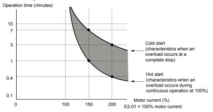
Figure 5.77 Protection Operation Time for General Purpose Motors at the Rated Output Frequency
