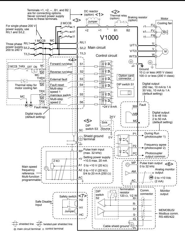
Figure 3.1 Drive Standard Connection Diagram
