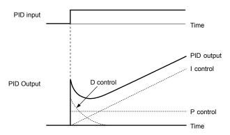
Figure 5.17 PID Operation
