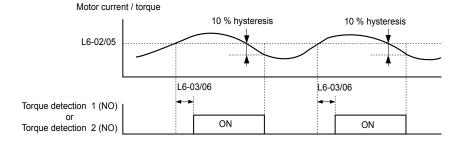
Figure 5.89 Overtorque Detection Operation
