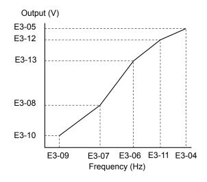
Figure 5.44 V/f Pattern for Motor 2
