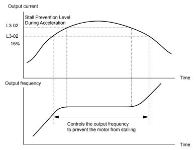
Figure 5.82 Stall Prevention During Acceleration for Induction Motors
