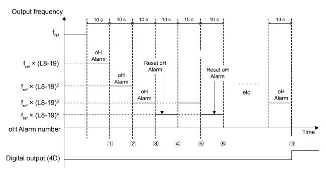
Figure 5.91 Output Frequency Reduction During Overheat Alarm
