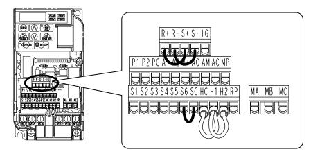
Figure C.9 Terminal Connections for Communication Self-Diagnostics
