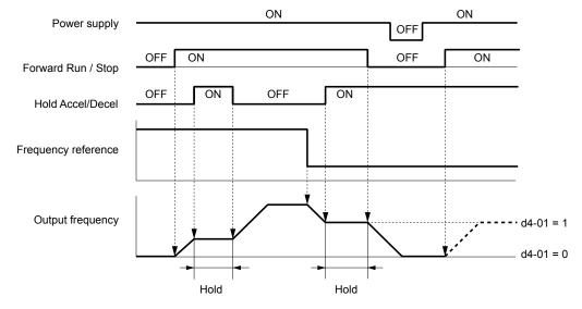
Figure 5.37 Frequency Reference Hold with Accel/Decel Hold Function
