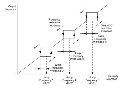
Figure 5.36 Jump Frequency Operation
