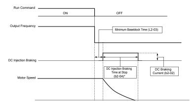
Figure 5.6 DC Injection Braking to Stop
