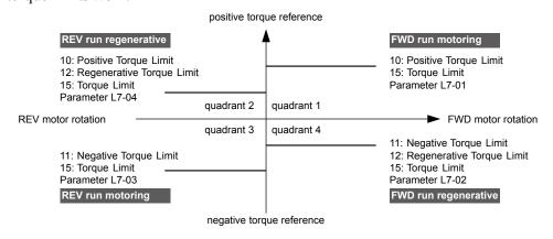
Figure 5.74 Analog Input Torque Limits
