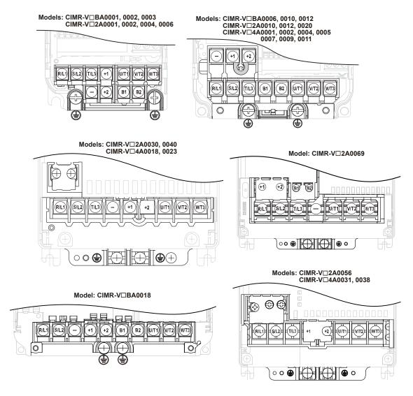
Figure 3.5 Main Circuit Terminal Block Configurations
