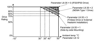
Figure A.2 Ambient Temperature and Installation Method Derating
