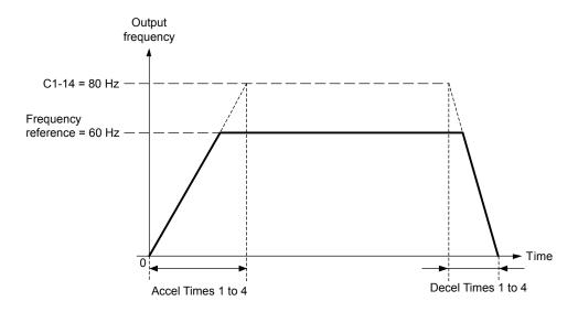
Figure 5.27 Accel/Decel Rate, Example 3 (C1-14 = 80 Hz, E1-04 = 60 Hz, Frequency Reference = 60 Hz)
