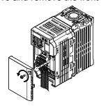
Figure 7.6 Remove the Front Cover
