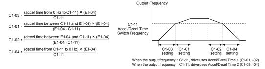
Figure 5.24 Accel/Decel Time Switching Frequency
