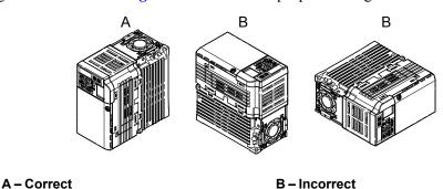
Figure 2.1 Correct Installation Orientation
