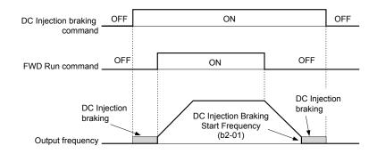
Figure 5.55 DC Injection Braking Input Timing Diagram
