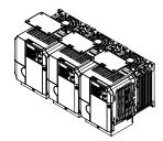
Figure 2.4 IP20/NEMA Type 1 Side-by-Side Mounting in Enclosure
