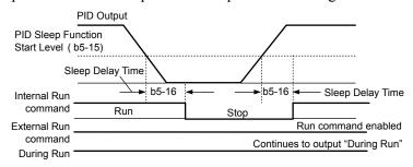
Figure 5.21 PID Sleep Operation
