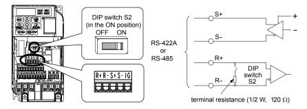
Figure C.5 Serial Communications Terminal and DIP Switch S2
