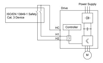
Figure D.11 Safe Disable Wiring Example
