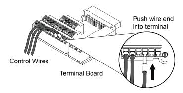
Figure 3.20 Connecting Wires to the Control Terminals
