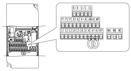
Figure 3.18 Removable Control Circuit Terminal Block
