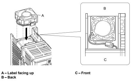
Figure 7.3 Cooling Fan Orientation
