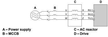
Figure 8.3 Connecting an AC Reactor
