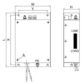
Figure D.7 EMC Filter Dimensions
