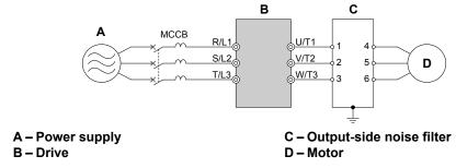
Figure 8.7 Output-Side Noise Filter
