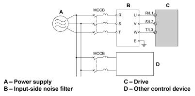
Figure 8.6 Input-Side Noise Filter (Three-Phase 200/400 V)
