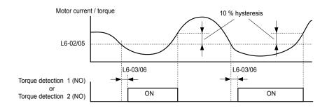
Figure 5.90 Undertorque Detection Operation
