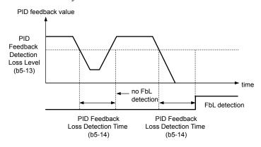
Figure 5.20 PID Feedback Loss Detection
