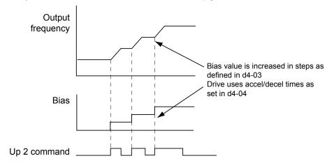
Figure 5.41 Up/Down 2 Bias when d4-03 > 0.0 Hz
