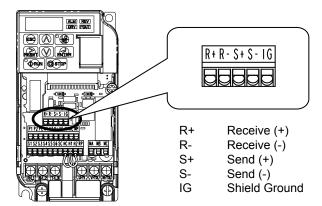
Figure C.2 Serial Communications Cable Connection Terminals
