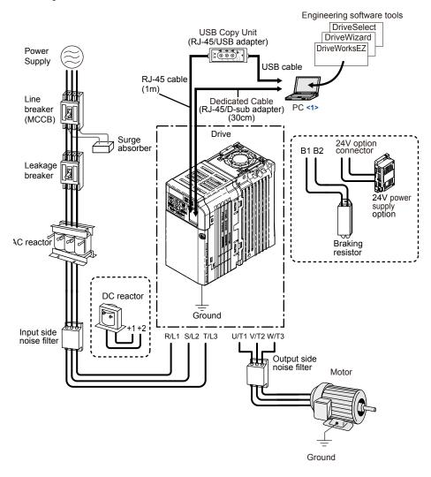
Figure 8.1 Connecting Peripheral Devices
