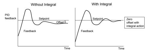
Figure 5.19 Offset Elimination by Integral Operation
