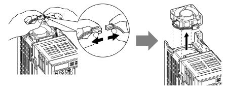
Figure 7.2 Disconnect and Remove the Fan
