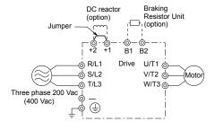
Figure 3.4 Connecting Three-Phase Main Circuit Terminals
