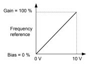
Figure 5.70 Analog Input A1 Default Characteristics
