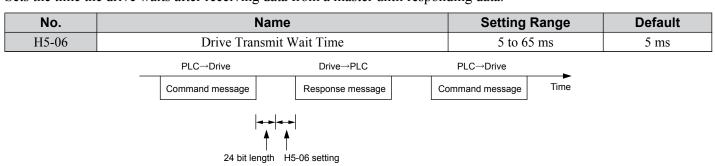
Figure C.6 Drive Transmit Wait Time Setting
