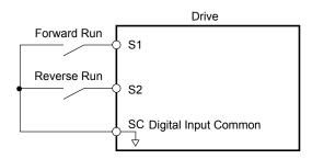
Figure 5.54 Example Wiring Diagram for 2-Wire Sequence
