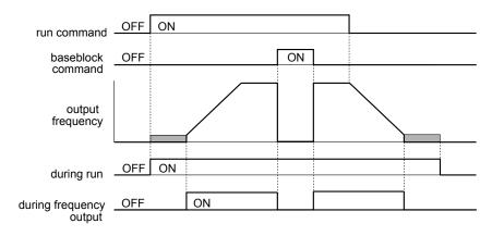
Figure 5.67 During Frequency Output Time Chart
