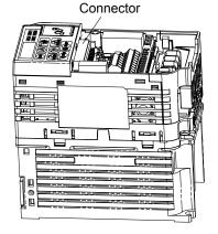
Figure 7.12 Terminal Board Reinstalled
