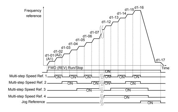
Figure 5.34 Preset Reference Timing Diagram
