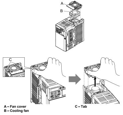
Figure 7.1 Remove the Cooling Fan Cover
