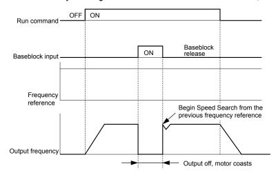
Figure 5.48 Baseblock Operation During Run
