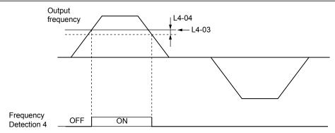
Figure 5.65 Frequency Detection 4 Example with Positive L3-04 Value
