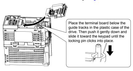
Figure 7.11 Terminal Board Reinstallation
