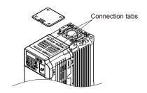
Figure 3.14 Reattaching the Top Cover
