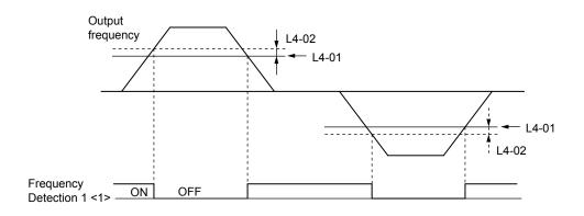
Figure 5.60 Frequency Detection 1 Time Chart
