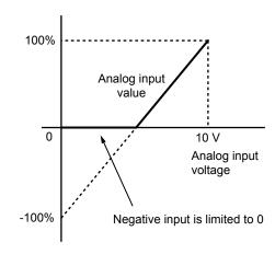
Figure 5.68 Analog Input with Limit (Bias Setting -100%)
