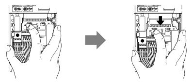
Figure 7.9 Remove the Terminal Board
