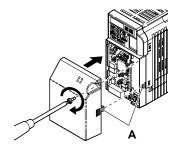
A -Align the tab with the mounting hole.
