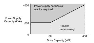
Figure i.3 Installing a Reactor
