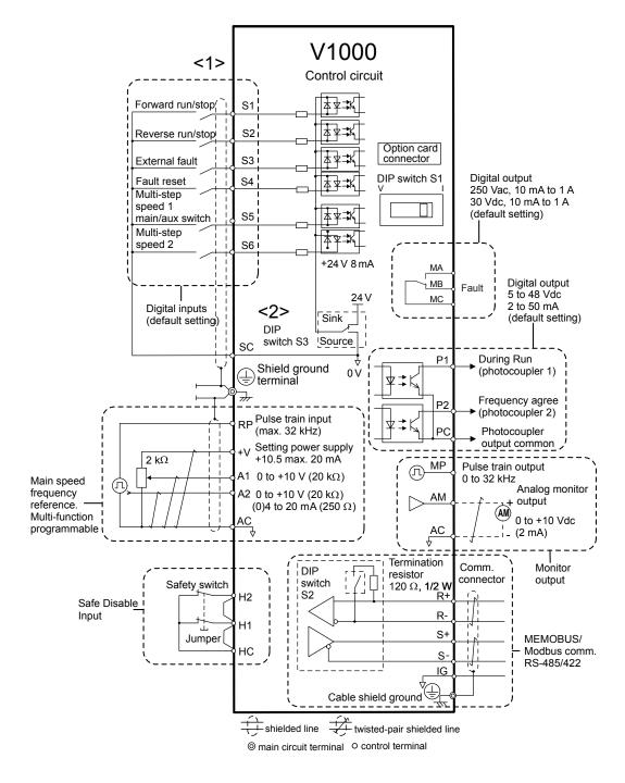
Figure 3.16 Control Circuit Connection Diagram
