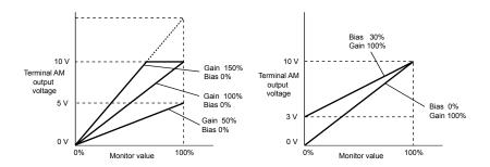
Figure 5.75 Analog Output Gain/Bias Setting
