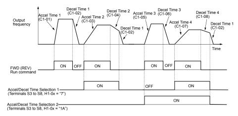
Figure 5.23 Timing Diagram of Accel/Decel Time Change
