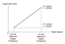
Figure 5.31 Adjusting ASR Proportional Gain and Integral Time
