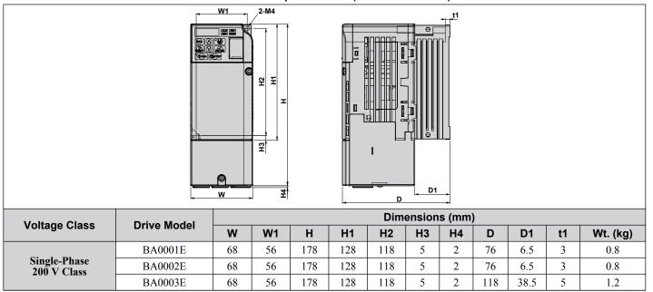
Table 2.6 IP20/Open-Chassis (with an EMC filter)
