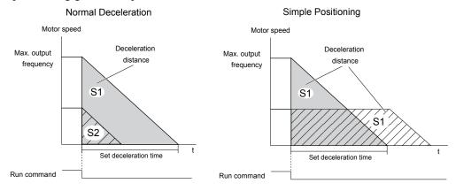
Figure 5.10 Simple Positioning Deceleration
