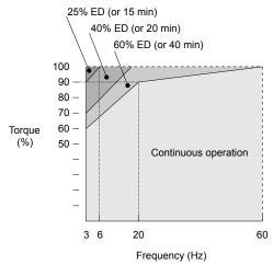
Figure i.4 Allowable Load Characteristics for a Yaskawa Motor
