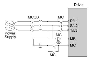
Figure 8.2 Connecting an MCCB
