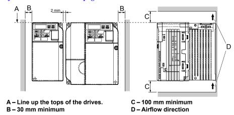
Figure 2.3 Space Between Drives (Side-by-Side Mounting)
