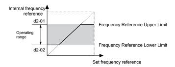
Figure 5.35 Frequency Reference: Upper and Lower Limits
