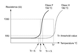
Figure 5.79 Motor PTC Characteristics
