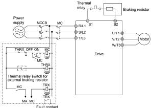
Figure 3.29 Connecting a Braking Resistor
