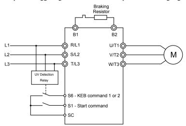
Figure 5.81 KEB Function Wiring Example
