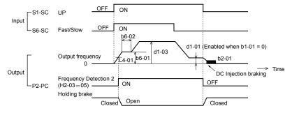
Figure 4.12 Holding Brake Time Chart
