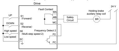
Figure 4.11 Brake Control Wiring
