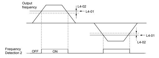
Figure 5.61 Frequency Detection 2 Time Chart
