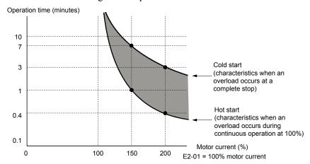
Figure D.9 Motor Overload Protection Time
