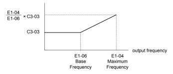
Figure 5.29 Slip Compensation Limit
