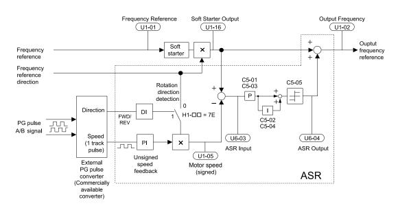
Figure 5.30 Speed Control with ASR in V/f with Simple Speed Feedback
