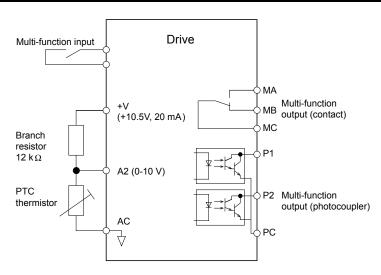
Figure 5.78 Connection of a Motor PTC
