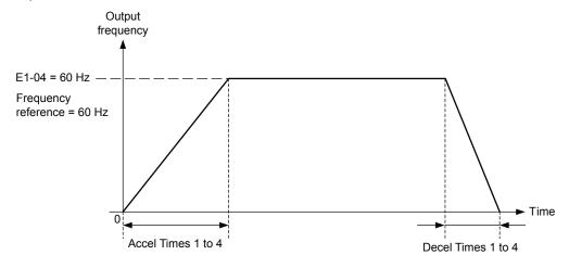
Figure 5.25 Accel/Decel Rate, Example 1 (C1-14 = 0 Hz, E1-04 = 60 Hz, Frequency Reference = 60 Hz)
