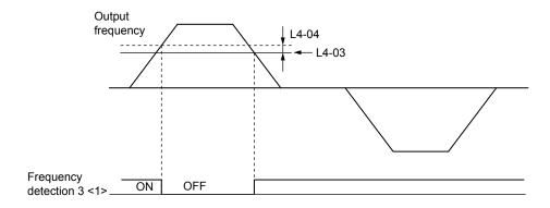
Figure 5.64 Frequency Detection 3 Example with Positive L3-04 Value
