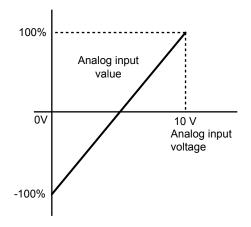
Figure 5.69 Analog Input without Limit (Bias Setting -100%)
