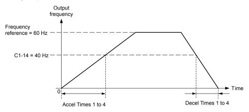
Figure 5.26 Accel/Decel Rate, Example 2 (C1-14 = 40 Hz, E1-04 = 60 Hz, Frequency Reference = 60 Hz)
