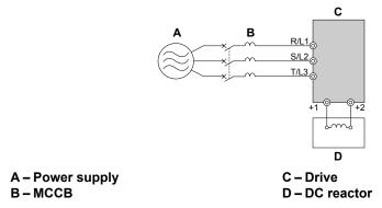
Figure 8.4 Connecting a DC Reactor
