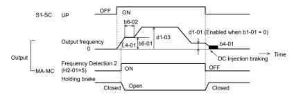
Figure 5.88 Holding Brake Time Chart
