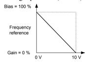
Figure 5.73 Frequency Reference Setting by Analog Input with Inverse Gain and Bias Settings
