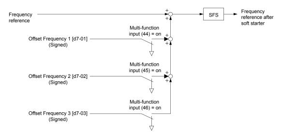
Figure 5.42 Offset Frequency Operation
