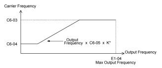
Figure 5.32 Carrier Frequency Changes Relative to Output Frequency
